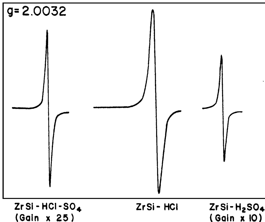
FIG. 3. Room temperature EPR signal of \text{ZrO}_2\text{-SiO}_2 sol-gel catalysts calcined at 400^\circ\text{C} in air.
